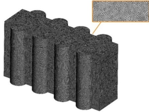
Figure 4. Unstructured Mesh Configuration
