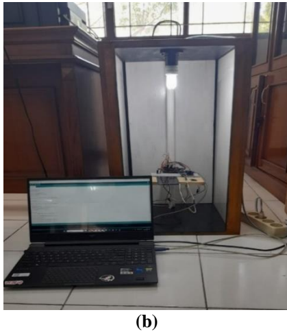
Figure 2. Scheme of the indoor photovoltaic system: (a) design, (b) implementation
