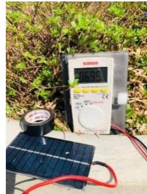
Gambar 14. Tegangan output maximal solar cell
