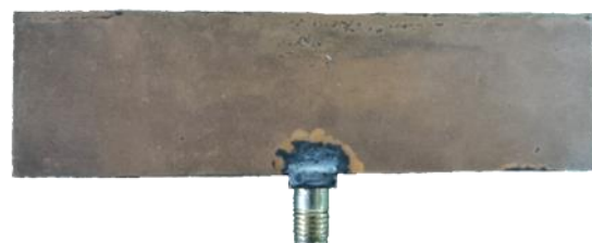
Gambar 10. Antena mikrostrip 1x4 tampak belakang
