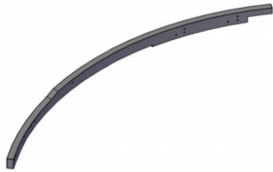
Gambar 7. Design Cam Safety Stretching Unit
