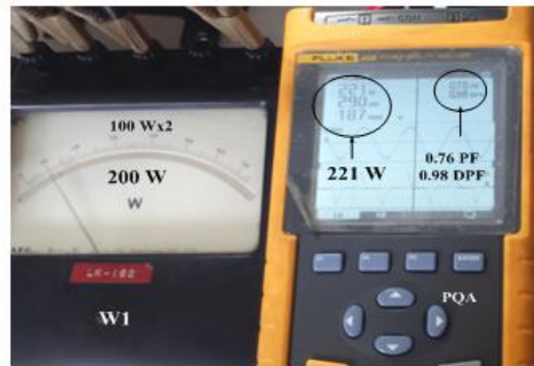
Figure 14. The difference in meter reading in LS18-1 test (all watt meter readings 10 x true value)
