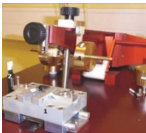
Gambar 3. Photography of ball-on-disc contact and tribotester system [14]
