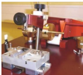
Gambar 3. Photography of ball-on-disc contact and tribotester system [14]
