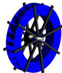
Gambar 4. Kincir overshot tampak samping
