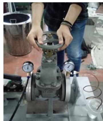
**Gambar 11. Proses pengujian kebocoran gate valve**
