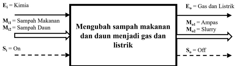
**Gambar 5. Blok fungsi biodigester tipe *fixed dome***
