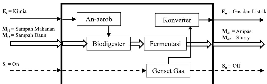
**Gambar 6. Diagram fungsi biodigester tipe *fixed dome***
