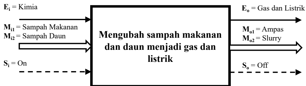
Gambar 5. Blok fungsi biodigester tipe fixed dome
