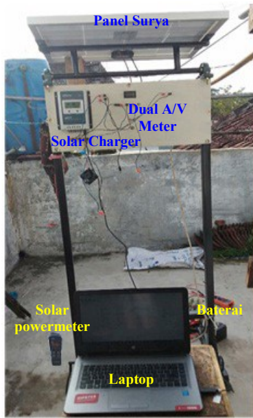
Gambar 2. Experimental setup pengujian trainer kit
