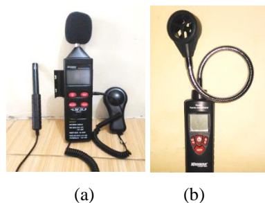
Gambar 5. Alat ukur: (a) 4in1 Environment Meter dan (b) Thermo Anemometer
