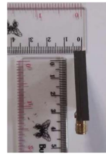
Gambar 13. Realisasi antena Mikrostrip Multilayer Parasitic U slot (a) Tampak Belakang (b) Tampak Depan (c) Tampak Samping
